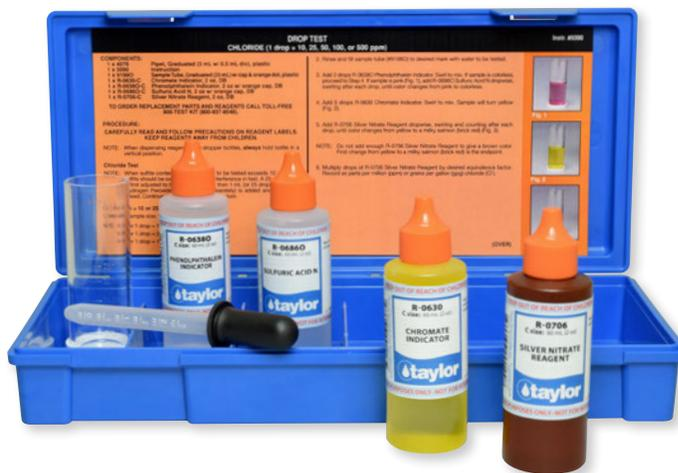
The K-1549 drop-test kit will perform 180 tests at 200 ppm.
