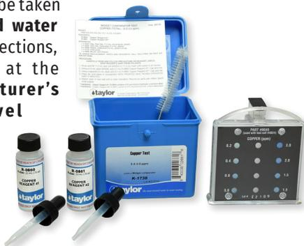
Matching the blue of the treated water sample to one of the eight liquid-color standards in the K-1738's Midget comparator is easy.
