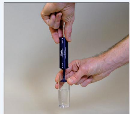
6. Carefully remove SampleSizer to avoid dragging out remaining water.
