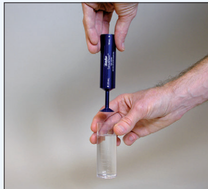
2. Orient SampleSizer for desired test volume: an arrow indicates the skinny end goes first for a 25 mL sample.
