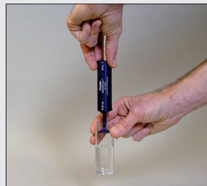
6. Carefully remove SampleSizer to avoid dragging out remaining water.
