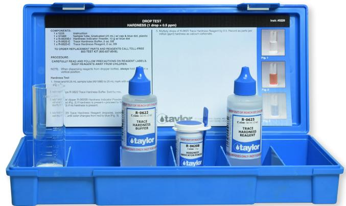
Taylor's hardness kits feature reagent caps color-coded to the instruction, plus a picture guide to the color transition in the titration (K-1504 pictured).
