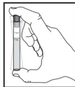
4. Secure stopper in test tube and shake for 5 seconds to mix.
